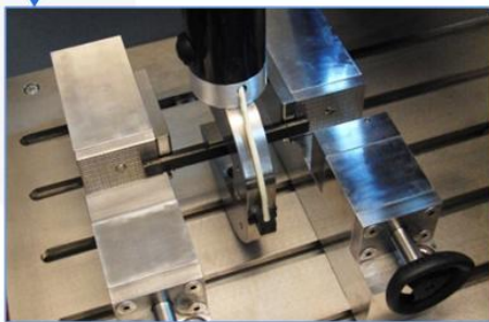
3-point bending 0.1 mm/s - 4.5 m/s
