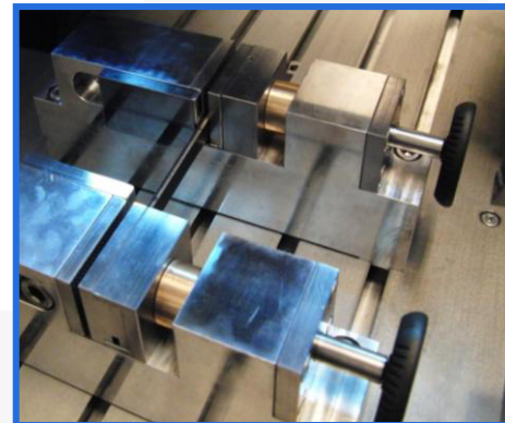
Fixed bending test
