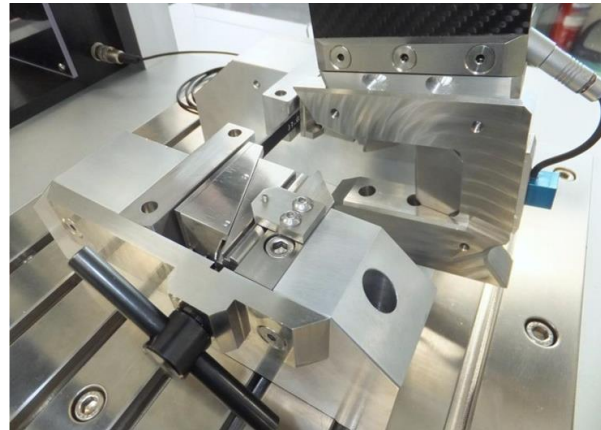
tension bending test
