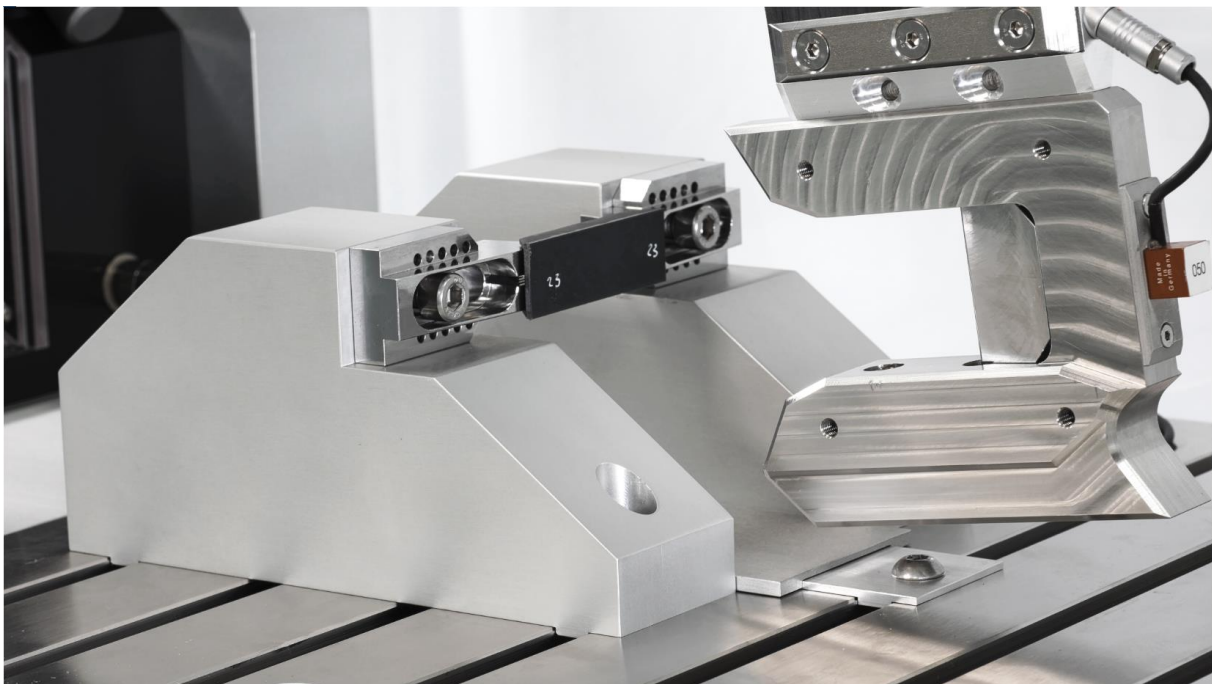
Figure 60: XX-Rib component test setup
